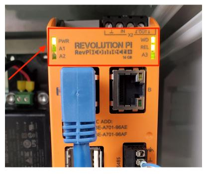
Communications status is indicated with the LEDs A1 and A2. After a few minutes, those LEDs should go from blinking to solid. If those LEDs are solid (not blinking), the system is communicating to the internet.
